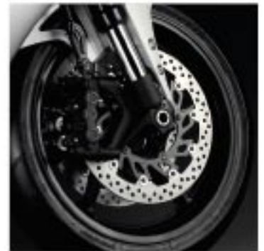
Bottom right: Six-piston caliper with lighter front brake
